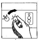
In systems with a room thermostat, set temperature selector at "7".
