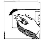
Set switch at 0. Clock of room thermostat stops running after approx. 70 h (power reserve).
